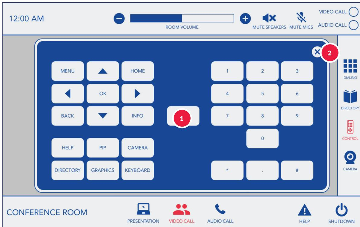
**1** Controls allowing for manual control of the codec for use while navigating through the codec’s on-screen display menus.
